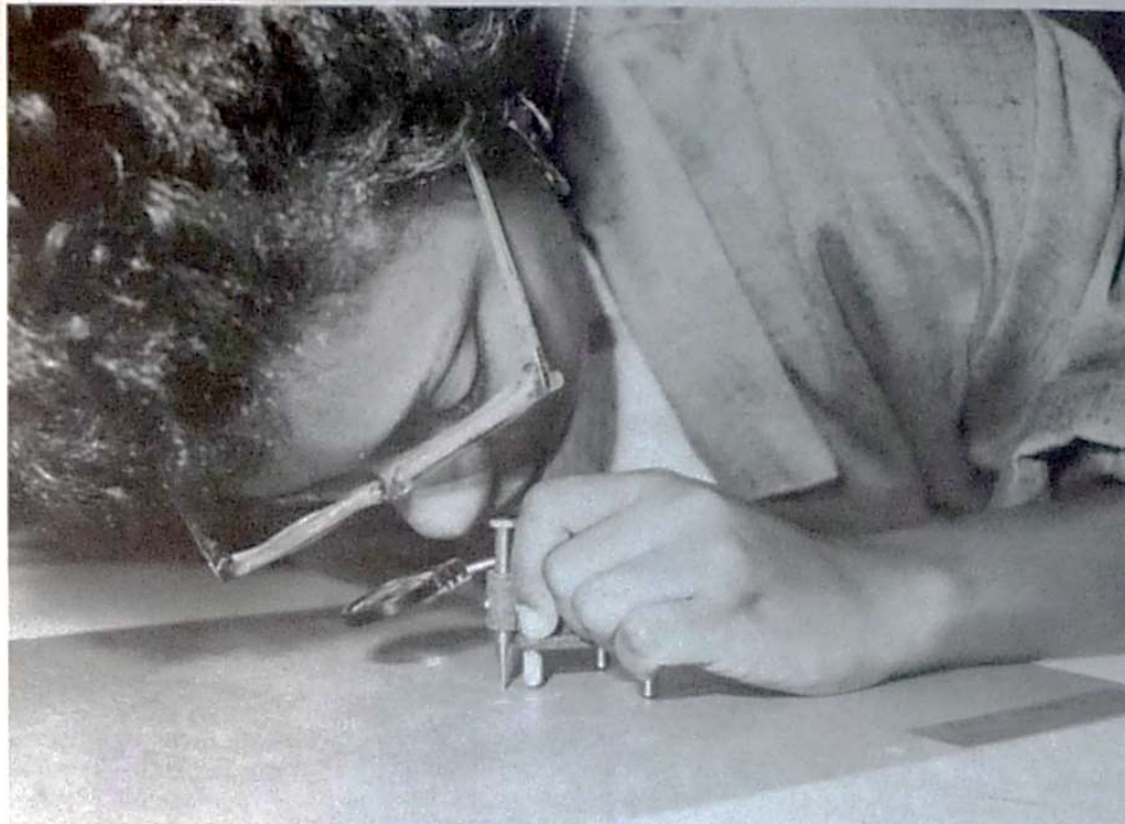
SXO cartographer Rhonda Neal scribes a negative during the mapmaking process at the San Antonio Office.
